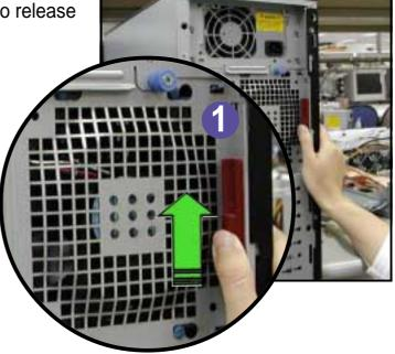
2. Slide the side cover for about half an inch toward the rear until it is disengaged from the chassis.
